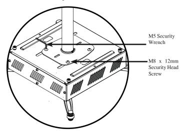
**Step 1.** Use the M5 security wrench and loosen the four (4) M8 x 12mm security screws.
